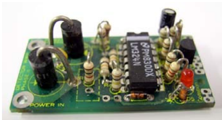
Integrated Signal Systems Block Occupancy Detector
